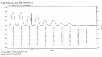
Fig. 1. Standard curve data for ammonium analysis using QuikChem Method 31-107-06-1-A.
